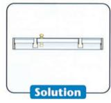
Box-construction sidelite door units are inherently weak and can rack, resulting in gaps and leakage. Our continuous sills and non-invasively routed headers cover the entire width of the door with one unbroken structure. This adds strength, preventing racking and alignment problems.
